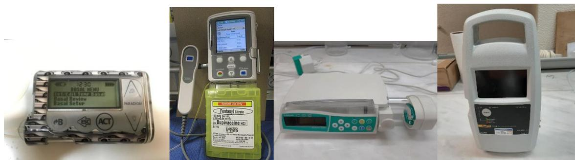
**Figure 3** – From left to right, insulin pump, a pain pump, a syringe pump and an infusion pump analyser
