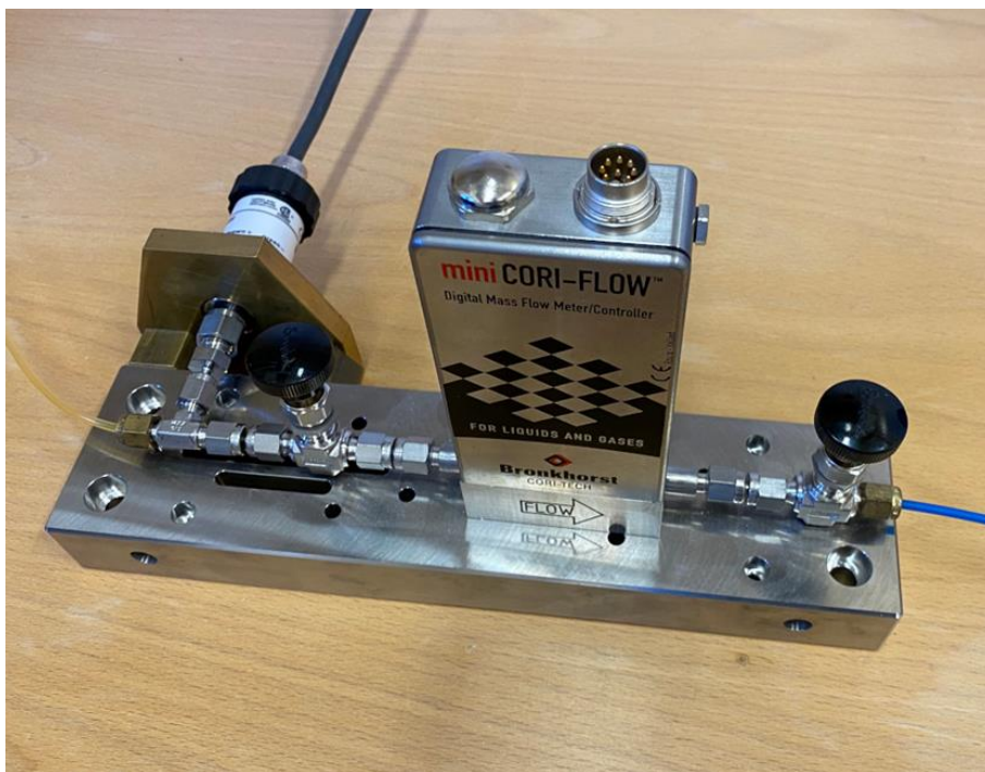
Figure 3.6.6 – Flow meter Bronkhorst M12 and pressure sensor (4...20 mA)
