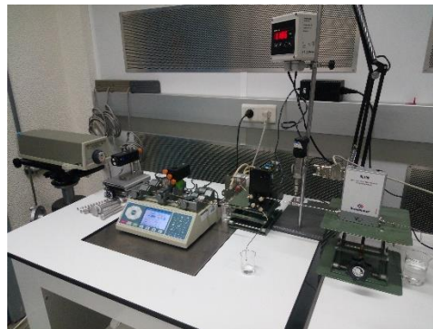
Figure 3.3.10 – Calibration of BL100 Bronkhorst meter using interferometry
