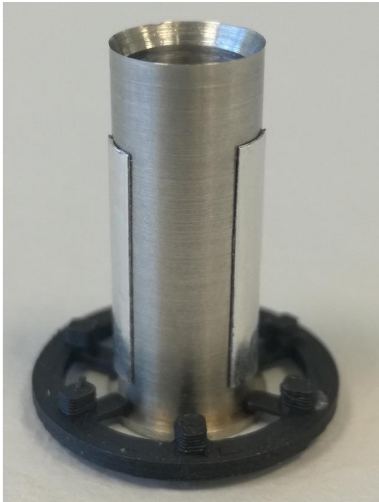
Fig. 3.2.2 - Prototype of the beaker; detail without the plexiglass lid and the tube (left), complete setup on a scale (right)
