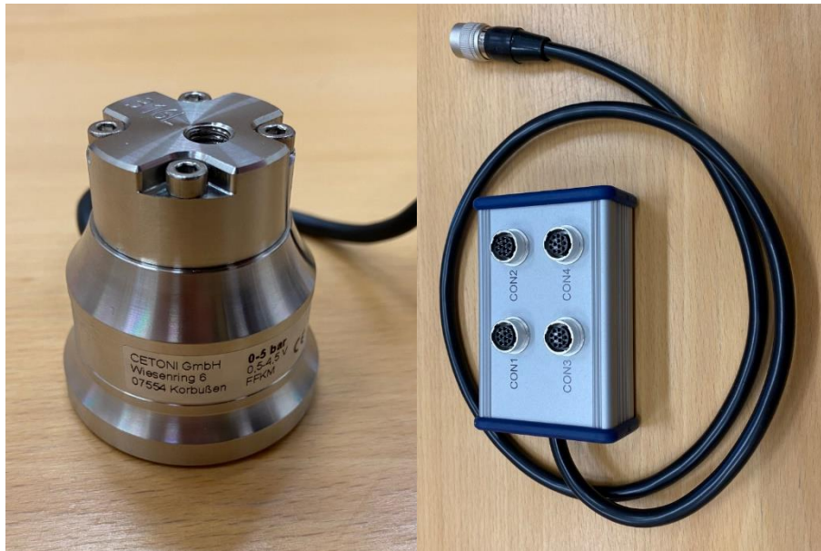
Figure 3.6.5 – Pressure sensor (pressure range 0-5 bar) and I/O distribution box
