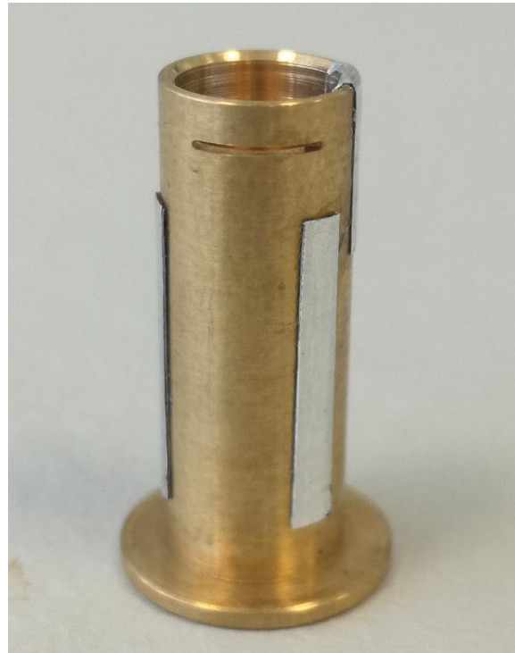
Fig. 3.2.2 - Prototype of the beaker; detail without the plexiglass lid and the tube (left), complete setup on a scale (right)
