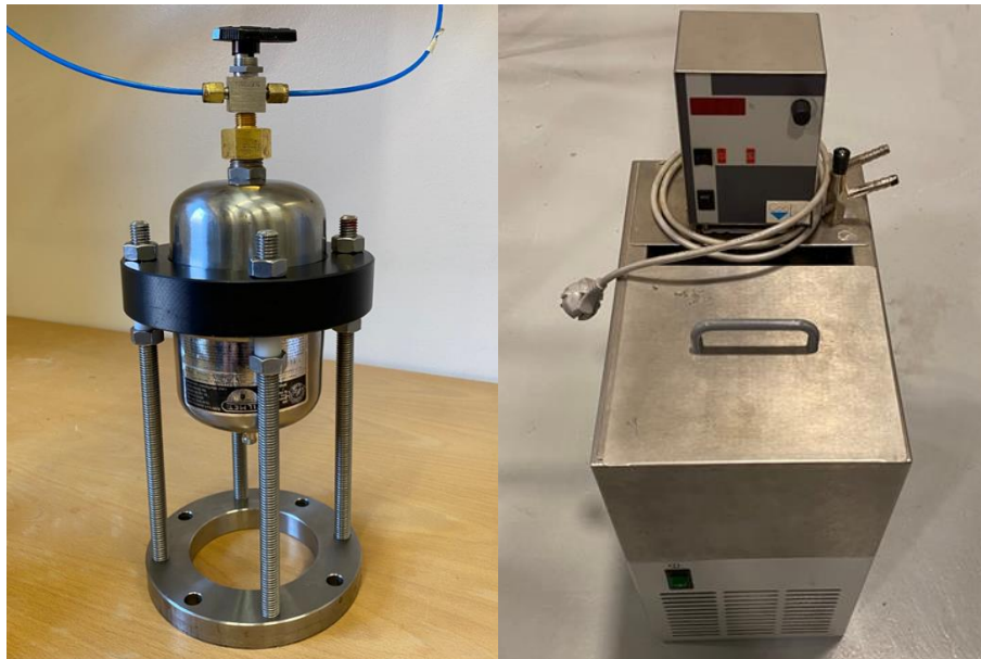
Figure 3.6.3 – Flow generator 3: Pressure vessel Zilmet (1 L, 10 barg max.) and temperature bath
